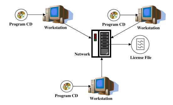
The network version is shipped on a single installation CD. On this CD are two items: the Visual Hydraulics setup program (Visual\_hydraulics\_setup.exe) and the license file for the network (VHlicense.dat). Note that your system administrator should install the program on the individual computers and the license file on the network per the steps below.
