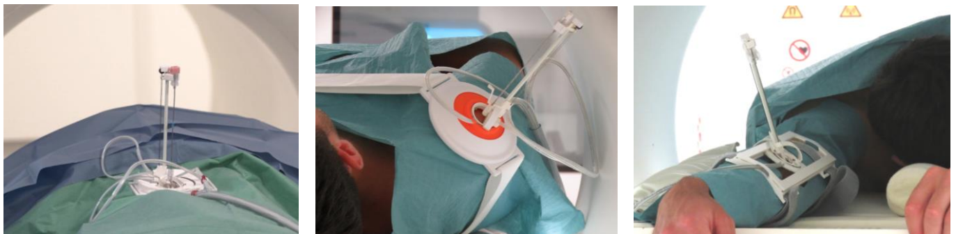
Fig. 1: Comparison of the differently configured IPUs installed on a planar- (left), spherical- (center) and cylindrical-IABM (right) in the according test scenario inside the MRI-tunnel: Left: Simulation of spine intervention; Center: Sim. of a shoulder-joint intervention; Right: Sim. of an elbow-joint intervention.
