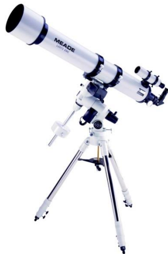
A Meade refractor with a German Equatorial Mount. Courtesy Greg Smye-Rumsby.
