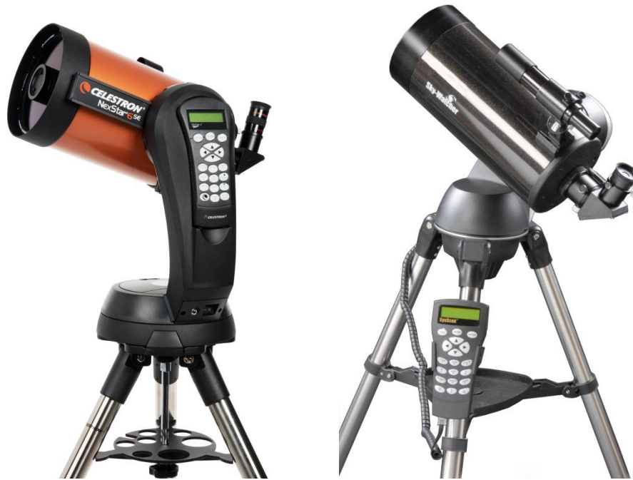
On the left is a Celestron Nexstar6 6" Schmidt-Cassegrain with go-to and on the right a Skywatcher Skymax-127 5" Maksutov with a SkyScan Go-to mount. Courtesy Greg Smye-Rumsby (left image) and Optical Vision Ltd (right image).
