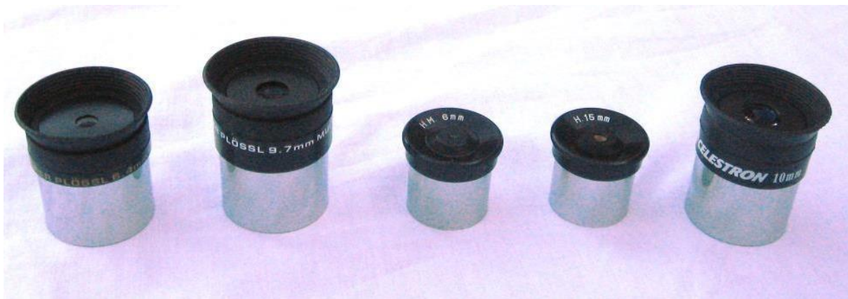
Range of eyepieces supplied with telescopes: on the left a 6.4mm and a 9.7mm “Super Plössl” by Meade; two 0.965” Huygens eyepieces (6 and 15mm) supplied with a cheap telescope; and a 10mm (Plössl?) eyepiece from Celestron.
