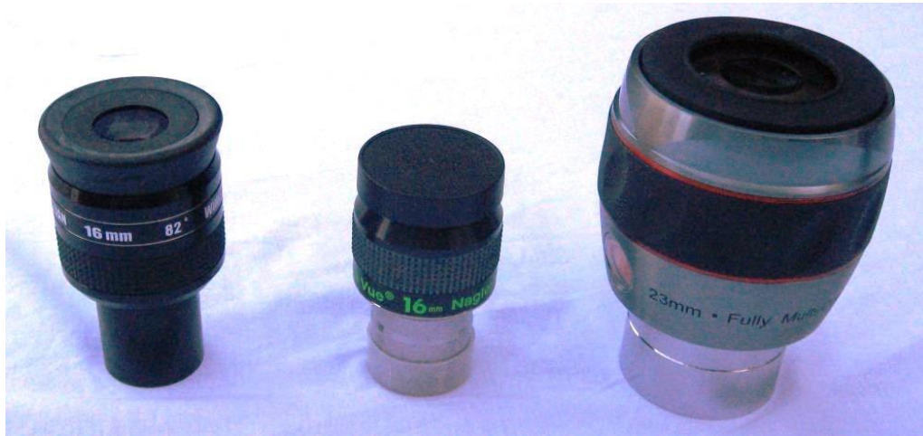
A selection of wide-angle eyepieces: the William Optics 16mm, the Tele Vue 16mm Nagler and the Celestron Axiom 23mm (now replaced by the Luminos range)
