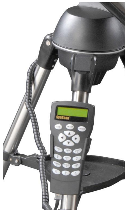
The go-to controller handset attached to the mount by a lead in the Skywatcher SkyScan go-to mount. Courtesy of Optical Vision Ltd.
