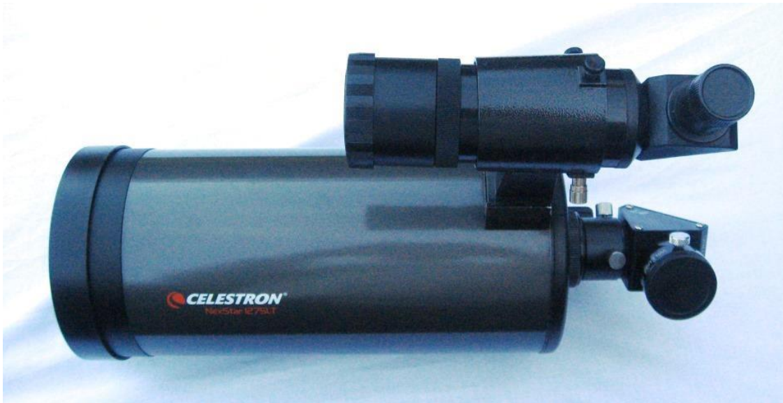
A Celestron 127 (5") Maksutov with an Orion (USA) right-angle finder and a William Optics star diagonal.
