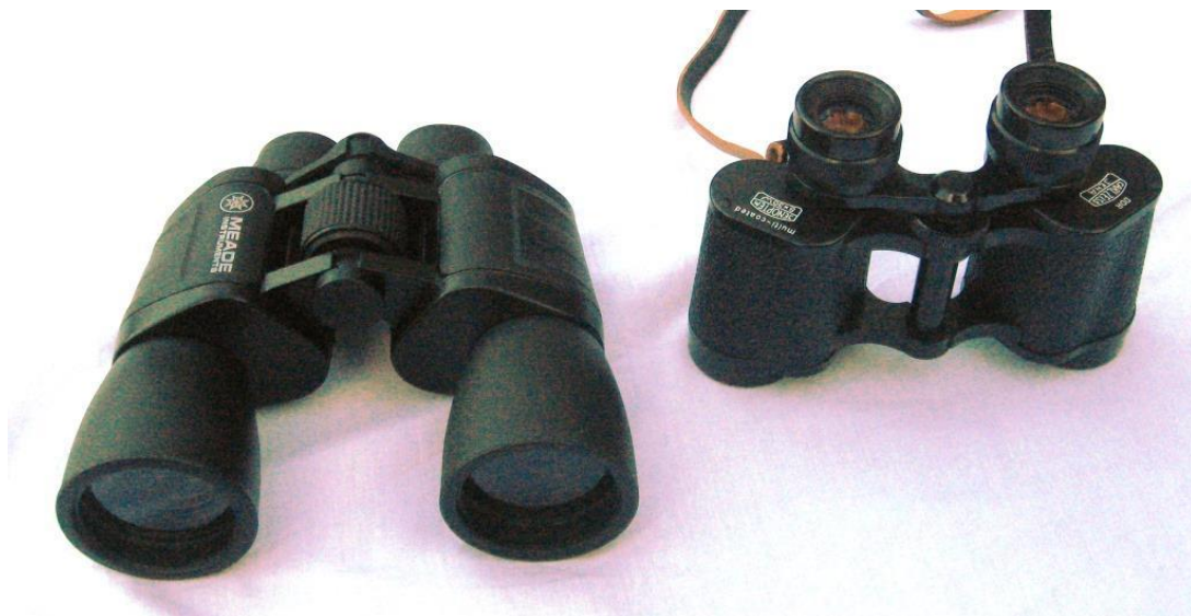
Two pairs of binoculars: Meade 10x50 and Carl Zeiss (DDR) 8x30
