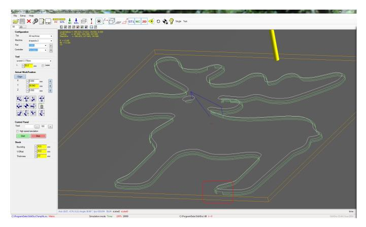
Figure 23: Visible in the marked rectangle is one of the tabs.
