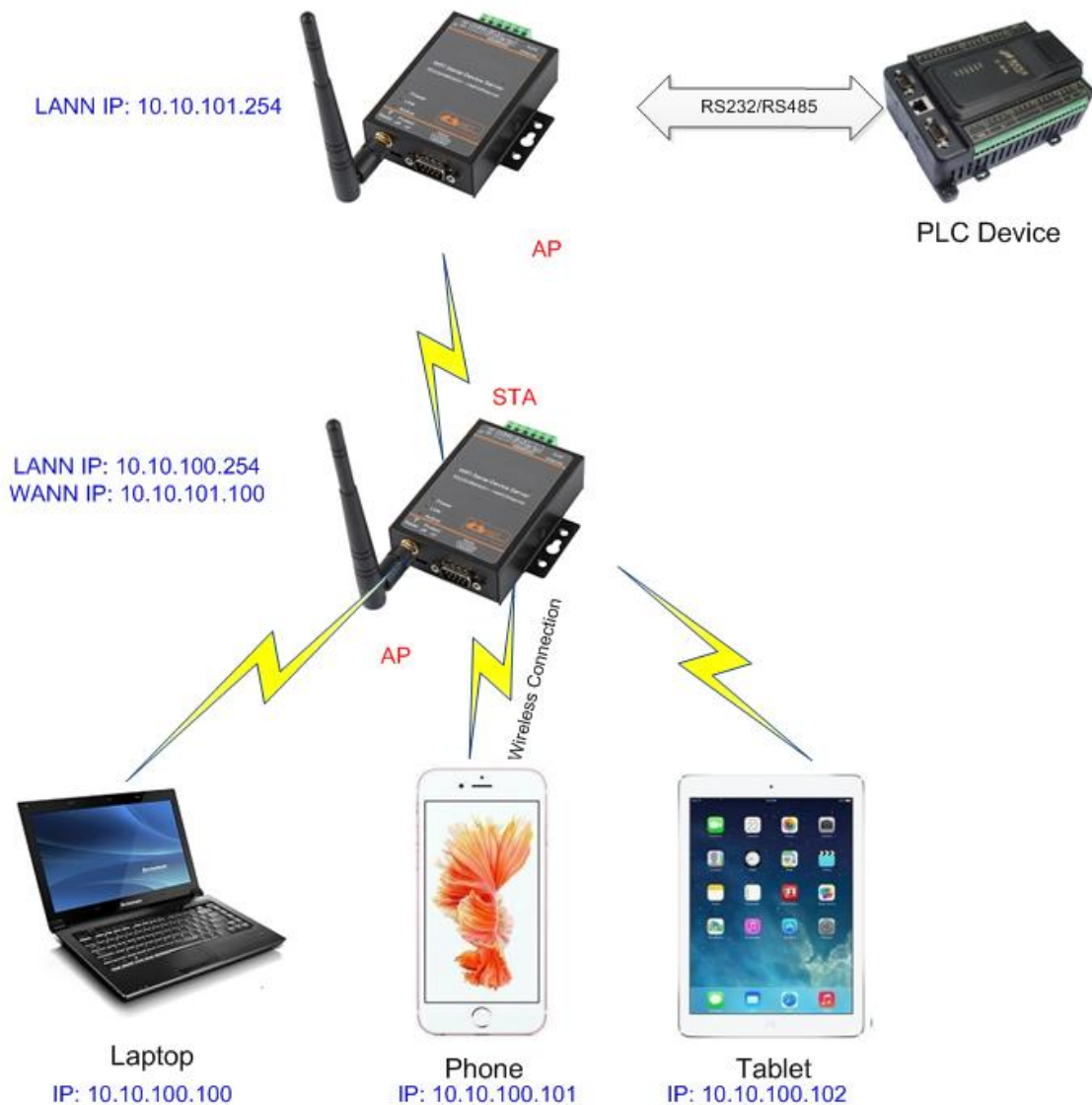
Figure 14. AP+STA Wireless Network
