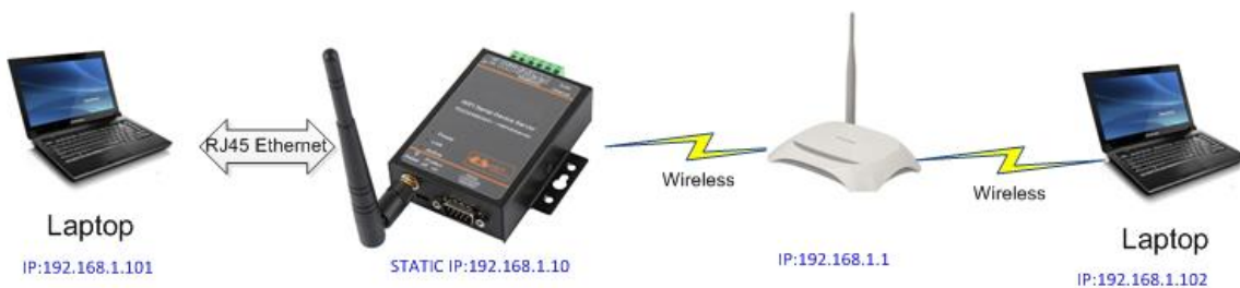
Figure 22. Ethernet Port Function(Bridge)
