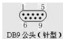
Figure 4. RS232 Pin Defination(Male/Needle Type)
