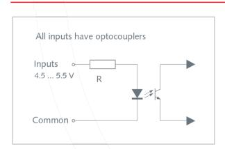
$R = 470 \Omega$ , excepted for the pulse input  $R = 220 \Omega$ .
