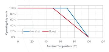
Values obtained with the motor screwed on an aluminum plate (dimensions 150 x 150 x 6 mm)
